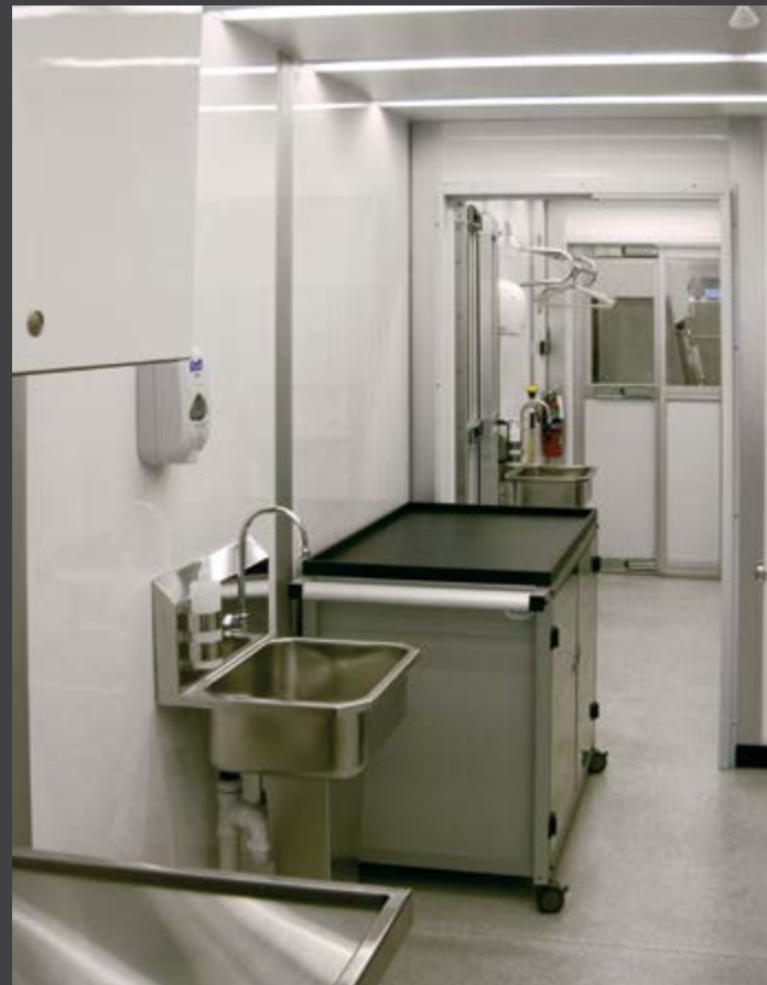
Medical Response Trailer, 3" Aluminum System & FRP Faced Wall Panels
