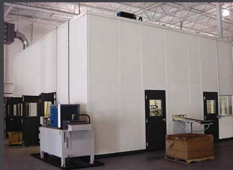
Tall enclosure with Soundstop Wall Panels
