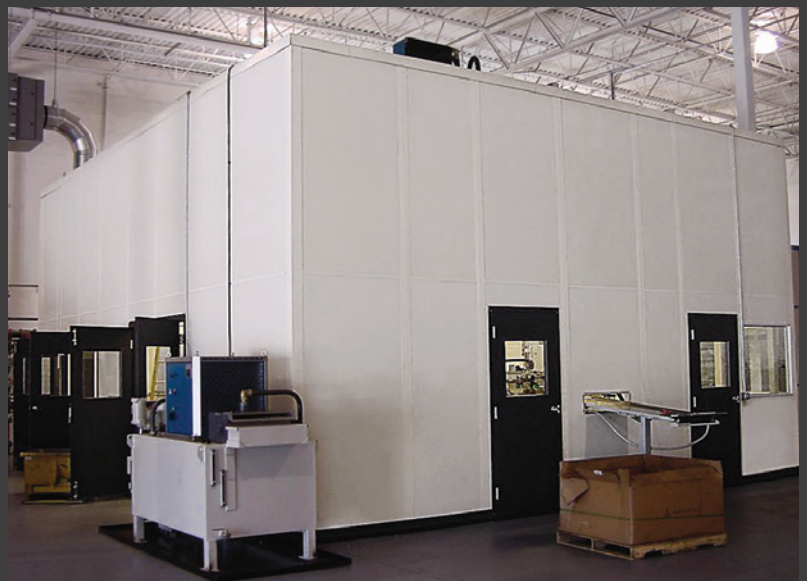
Tall enclosure with Soundstop Wall Panels
