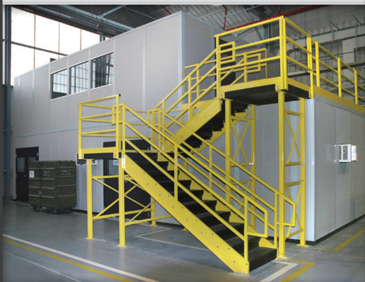
Second story in-plant office over in-plant shop; utilizing InPlant's 3\"
