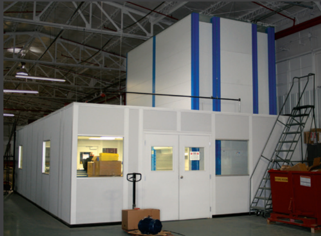
Environmentally controlled enclosure to ensure production quality
